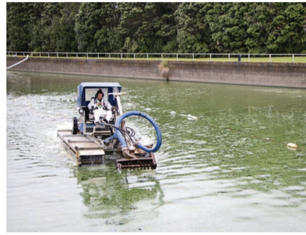
An amphibious Truxor vehicle gets to work in the NPDC Waste Water Treatment Plant sludge lagoon.
